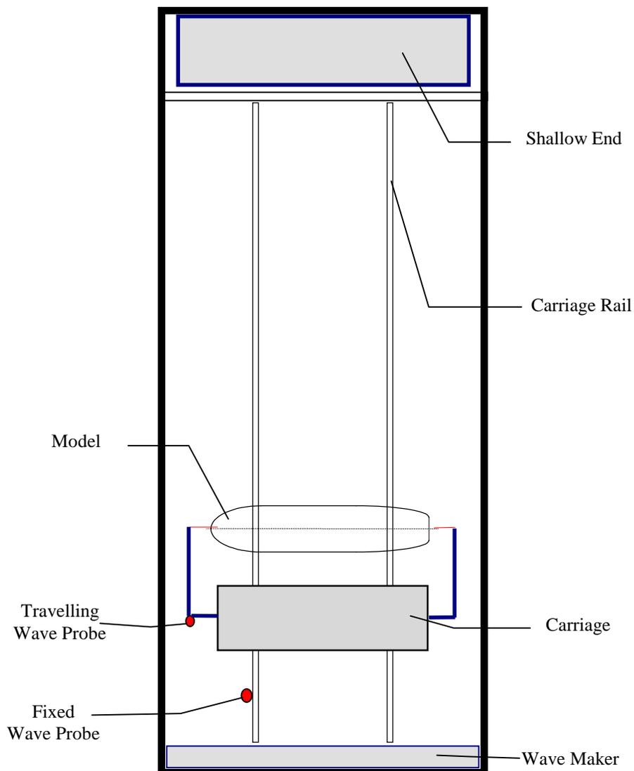
Figure 6: The Model Test method – Experimental Set-up
