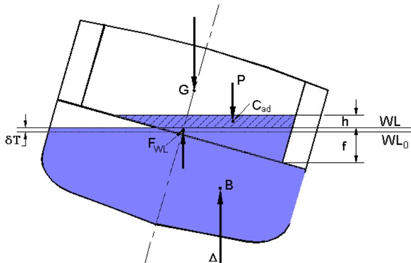
**Figure 4:** Stability of a Damaged Ship with Water Accumulated on Deck
